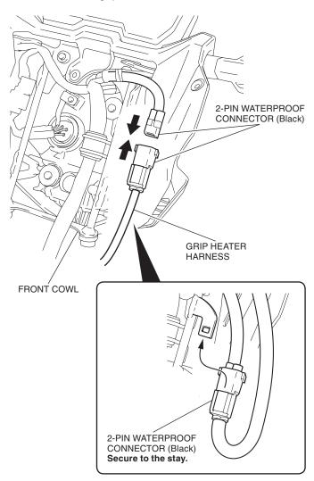
59. Secure the grip heater harness with the wire tie as shown.
