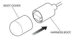
44. Secure the boot cover with electrical tape as shown.
