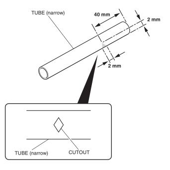
30. Pass the cut tube over the grip heater harness as shown.
