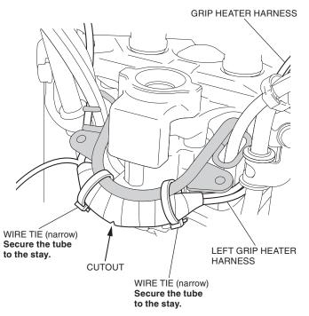
56. Secure the left grip heater harness and grip heater harness as shown.
