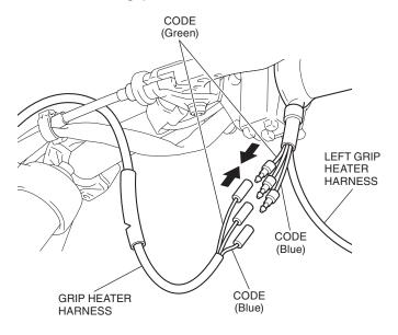
32. Slide the cut tube as shown.
