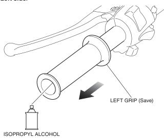
21. Using a isopropyl alcohol, remove all traces of adhesive from the left handlebar.
