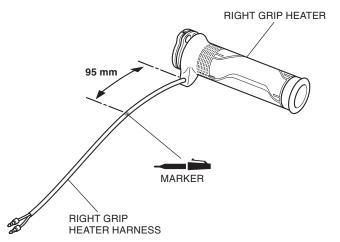
12. Install the clip band on the marked position as shown.
