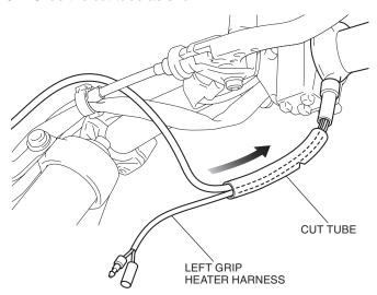
33. Secure the tube with electrical tapes as shown.
