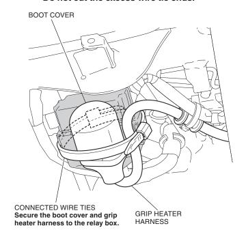
48. Secure the grip heater harness with the wire tie as shown.
