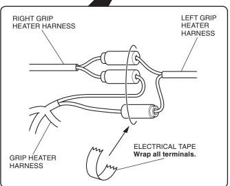
39. Wrap the right grip heater harness and grip heater harness with electrical tape as shown.
