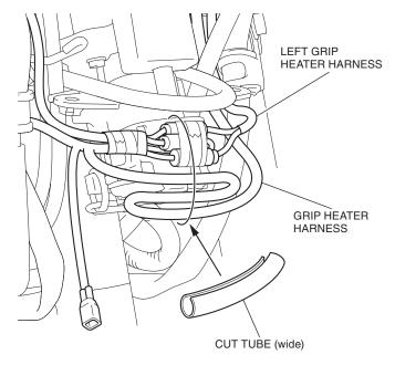
53. Secure the tube with electrical tapes as shown.
