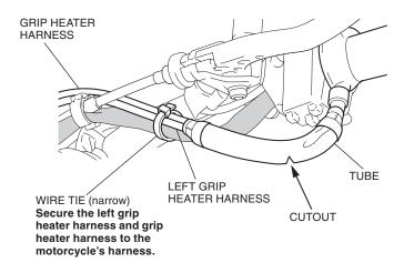
50. Secure the right grip heater harness with the clamp as shown.
