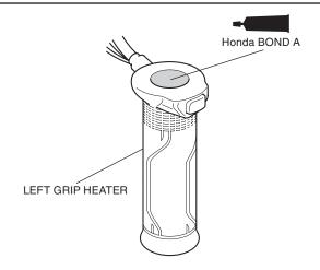
23. Apply Honda Bond A to the left handlebar as shown.
