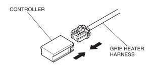
42. Fit the harness boot over the controller as shown.
