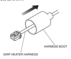
41. Connect the controller as shown.
