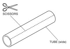
52. Cover the harness with the cut tube as shown.
