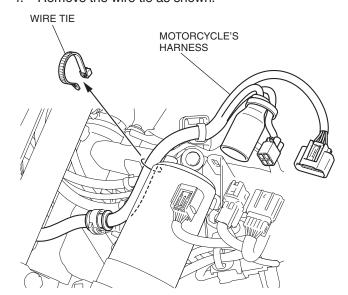
5. Release the clip band and clip as shown.
